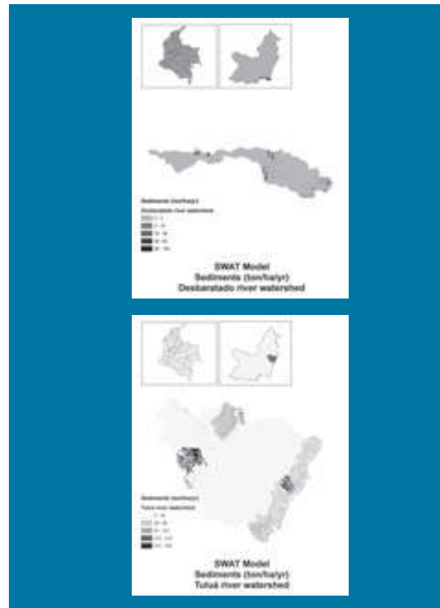
Figure 7. SWAT Model: Estimation of sediments for the watersheds of the Desbaratado and Tulua rivers, Cauca Valley, Colombia. Water for Life Water Fund. • Source: CIAT, Feasibility Study. Water for Life Water Fund, 2009.
